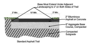
Typical Asphalt trail details; Source: DBPT
