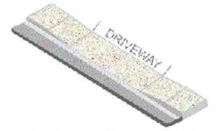
Conditionally Acceptable – The "tip" at the driveway apron allows for safer passage with no cross-slope.
