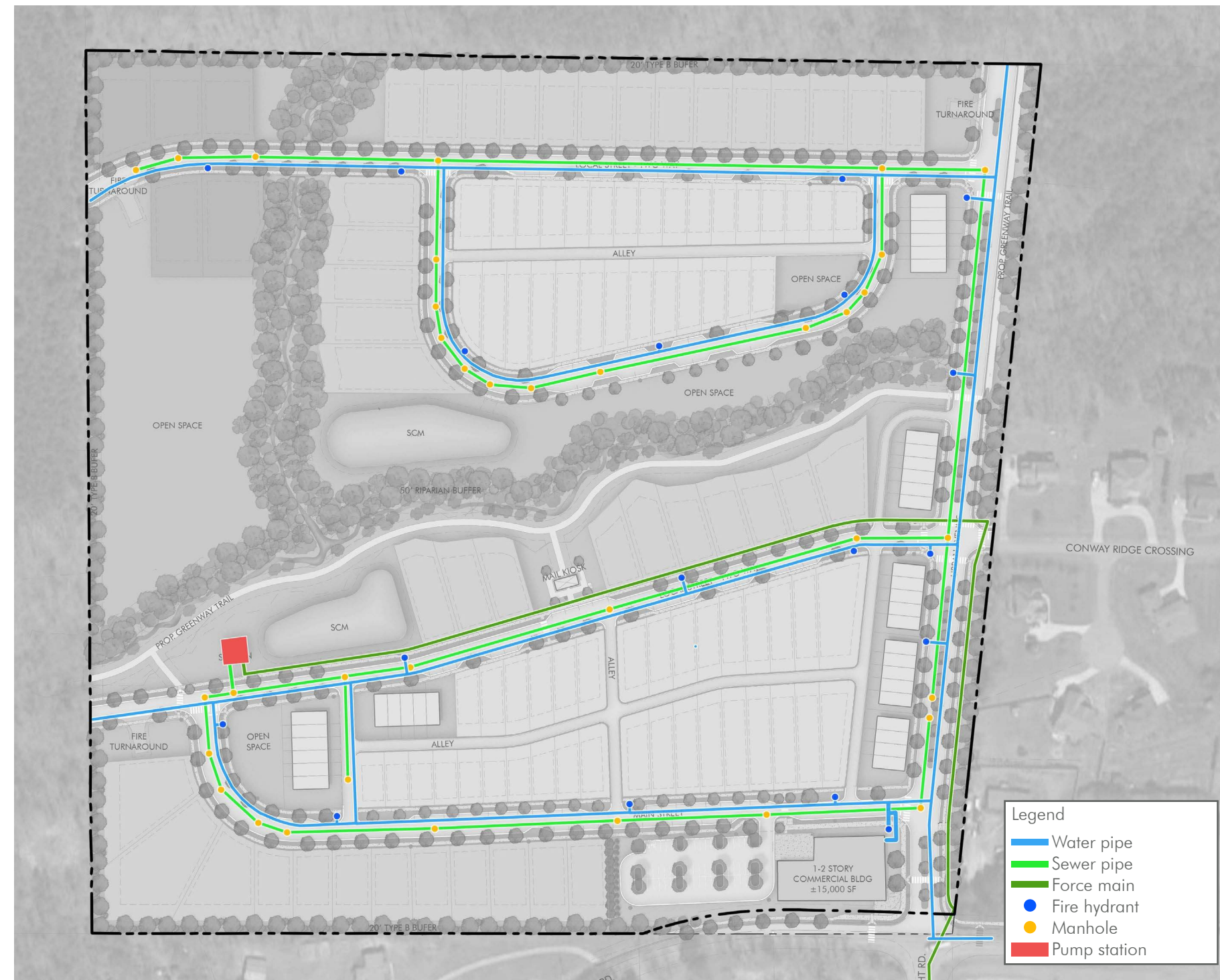
Figure 14: Weldon Preliminary Utility Plan
