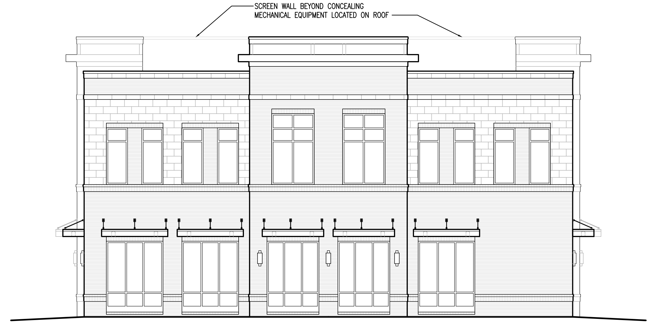
BUILDING 3: EAST ELEVATION SCALE: 1/8" = 1'-0"
