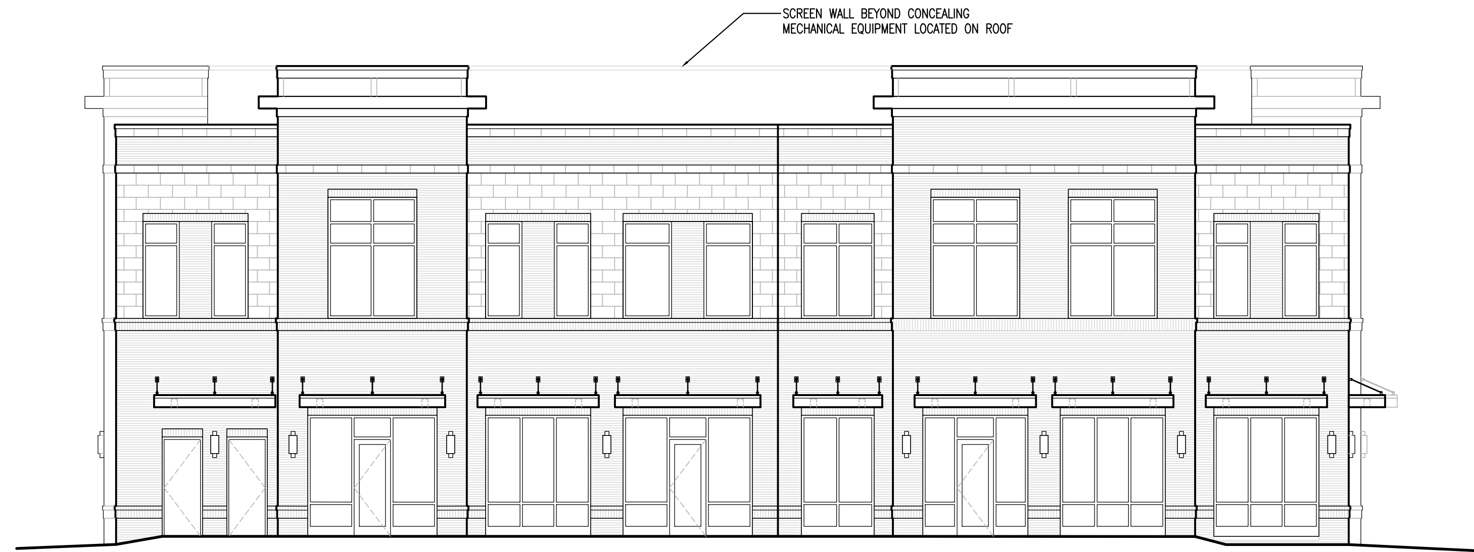
BUILDING 3: NORTH ELEVATION SCALE: 1/8" = 1'-0"
