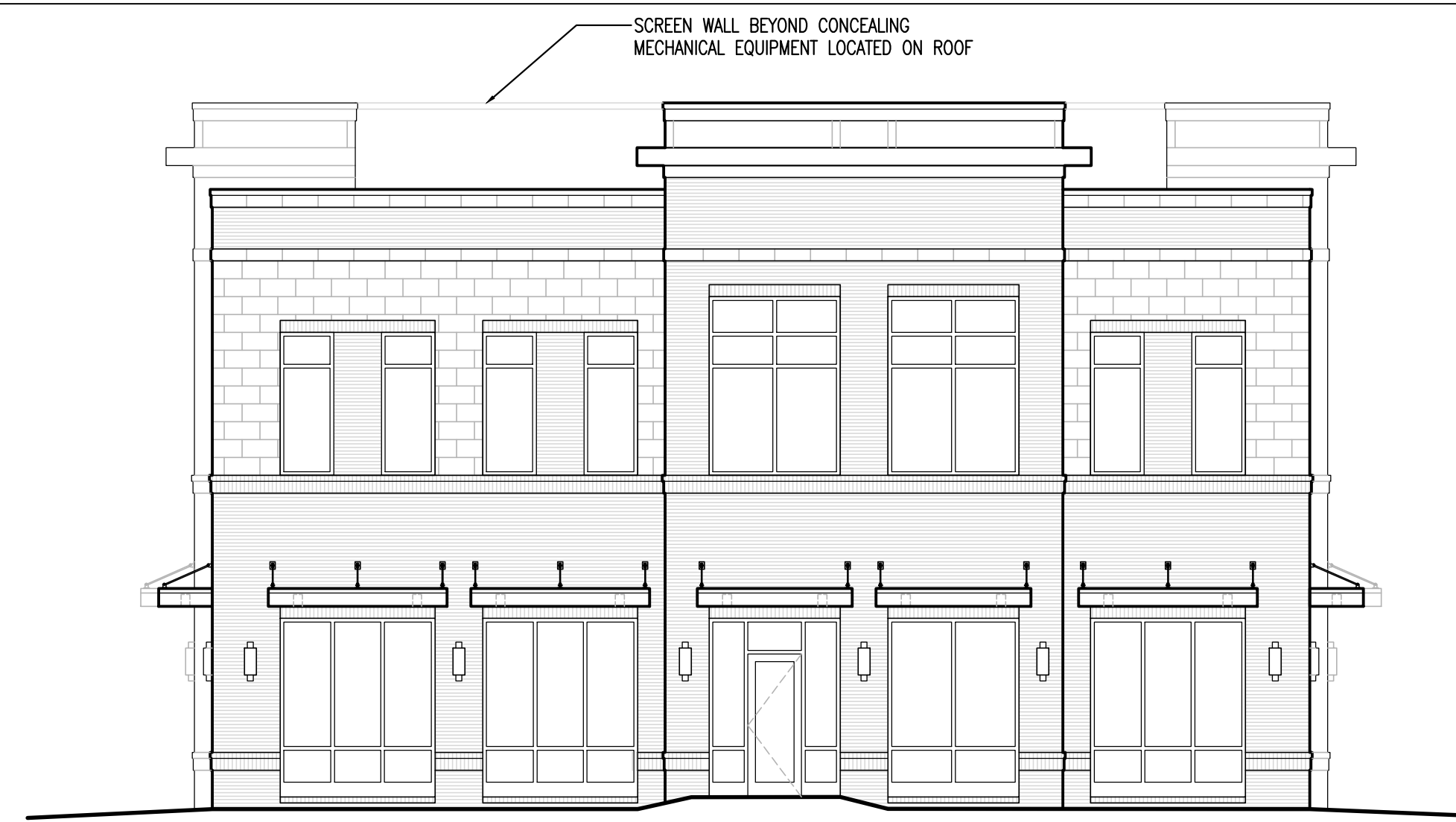
BUILDING 2: WEST ELEVATION SCALE: 1/8" = 1'-0"
