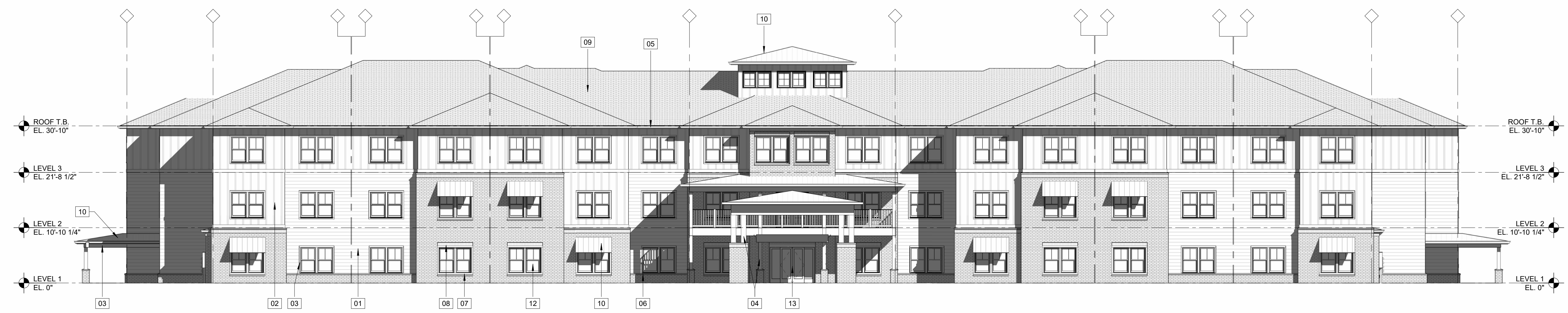
1 EXTERIOR ELEVATIONS (BUILDING TYPE "II") A107/A303 3/32" = 1'-0"
