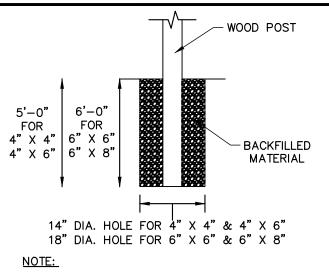
TREATED WOODEN POST SHALL BE PLACED IN PRE-DUG HOLE IN GROUND. BACKFILLED USING SUITABLE MATERIAL. AND TAMPED THOROUGHLY TO PROVIDE A RIGID SUB-SURFACE CONDITION AROUND THE POST.
