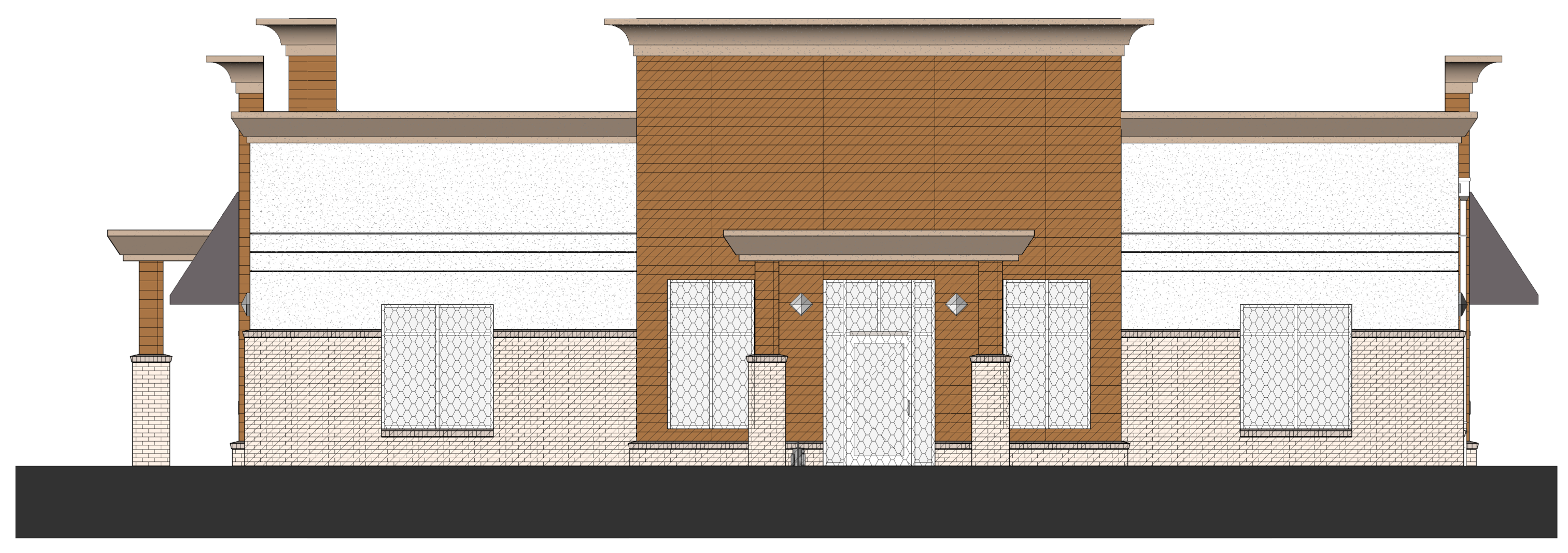
3 MCKNIGHT DRIVE ELEVATION SCALE: 3/16" = 1'-0"
